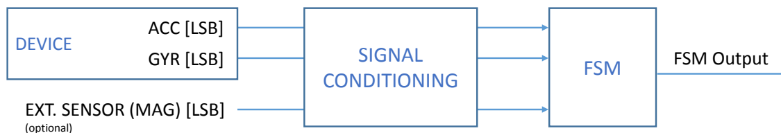
Figure 2. State machine in the LSM6DSRX
