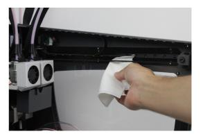
**11.** Apply the lubricating oil pencil along the linear guides of the X and Y axes, with special emphasis on their superior and inferior faces. Make sure there is no excess oil dripping.
