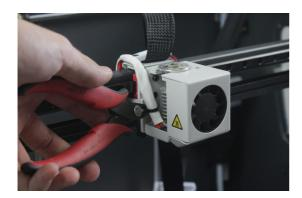
**9.** At the back of the toolhead carriage, press the connector to remove the cable of the hotend.
