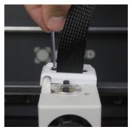
13. Insert the teflon tube until it stops, making sure it is well placed. Put back the black clip and the black piece.
