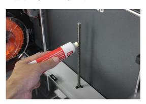
**6.** Turn on the Sigmax and from the LCD screen, go to *Utilities --> Maintenance --> Move printing surface.* Raise and lower the platform twice to evenly distribute the oil and grease. Finally, remove the remnant grease.
