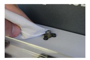
**7.** Once the process for the Z axis is finished, let's clean and lubricate X and Y linear guides. First of all, turn off the Sigmax. During this process it's recommended to manually move the axes in order to reach all the guide.
