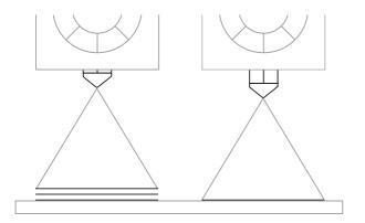
The Sigmax automatically corrects the offsets when printing in Duplication/Mirror modes. However, this correction distorts the first layer of the model by repeating it as many times as needed.
