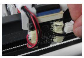
10. Remove the old hotend and place the new one, connecting it at the back of the toolhead carriage.
