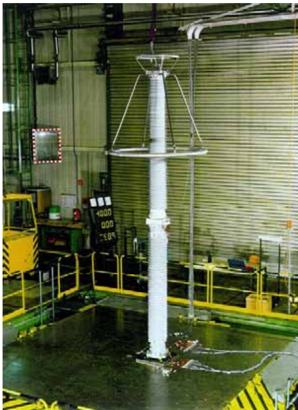
Fig. 22: Polymer housed arrester for a 550-kV-system during seismic testing on a shaking table
