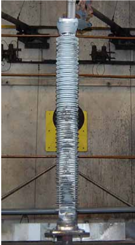
Fig. 24: Polymer-housed arrester ("tube design") after a test at rated short-circuit current (80 kA, 200 ms). The housing has remained completely intact.
