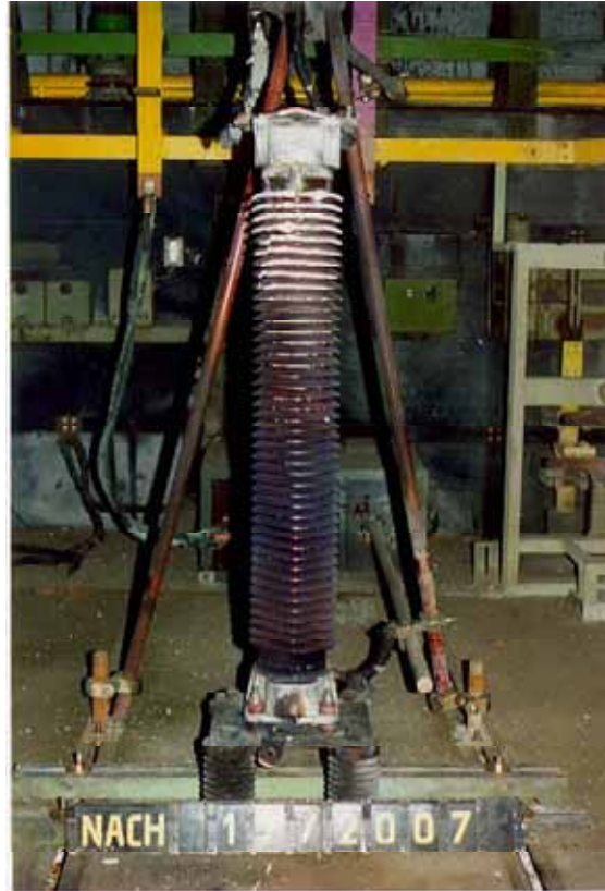
Fig. 25: Porcelain-housed arrester after a test at rated short-circuit current (63 kA, 200 ms). Apart from a few broken sheds, the housing has remained intact.
