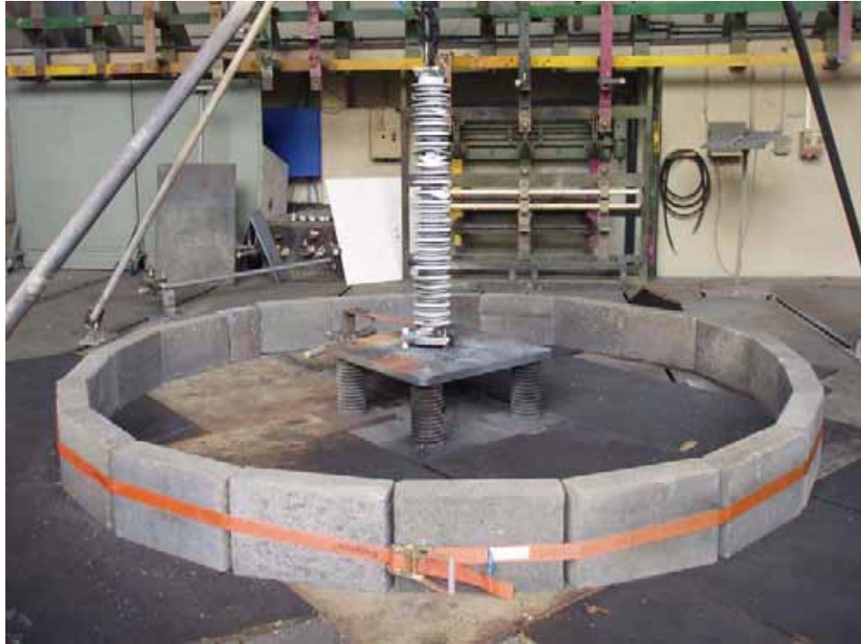
Fig. 23: Polymer-housed arrester ("tube-design") after a short-circuit test at rated current (65 kA, 200 ms). The housing is ripped but in mechanically sound condition. Details of the test setup can well be seen. For further information see short-circuit tests in the appendix.
