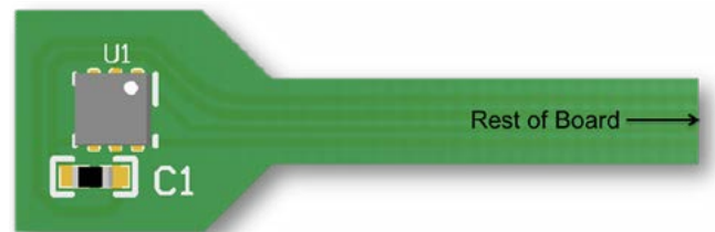
Figure 1. The TMP117 (U1) on a flexible PCB. Using an extended arm isolates the integrated circuit from heat generated by other devices.
