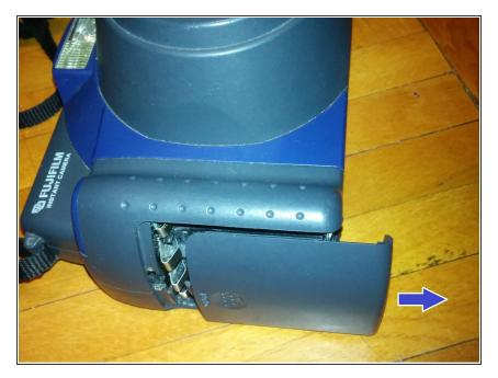
First, push on the recessed part of the battery cover while sliding it away from the camera to remove it. Then, remove all the batteries from the camera.
