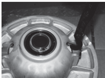
Insert hooked end of tool.
