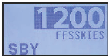
Figure 3004. (Sheet 1 of 1) Reverse Video Examples when KGX Control Panel is in External Control Mode
