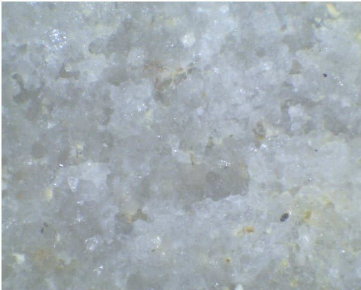
Quartzite at 30x Magnification – Note fusing of grains, low appearance of grain structure, more massive appearance and glassy texture; Other quartzite sample may exhibit a more coarse grained structure, but grains would be fused, with glassy texture and samples would fracture predominantly through grains as opposed to along grain faces.
