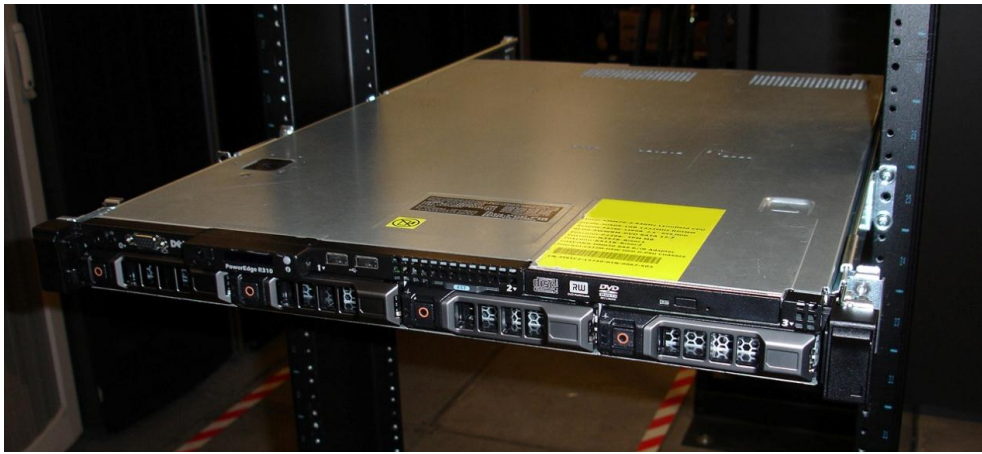
Figure 12. R415 Mounted in A4 Static Rails (2-Post Center Mount Configuration)
