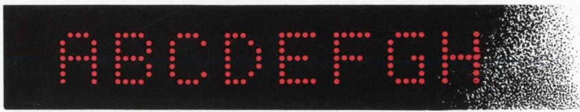
16/18 Character Position Panel, 5 x 7 Dot Matrix, Characters 0.4" High. Available as numeric only or alphanumeric panel with 64-character format.
