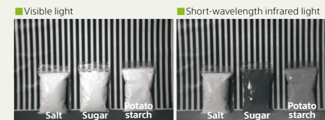
Photos of salt, sugar, and potato starch in visible light and short-wavelength infrared light. Certain differences that are hard to distinguish in visible light can be identified based on different absorption rates of short-wavelength infrared light.
