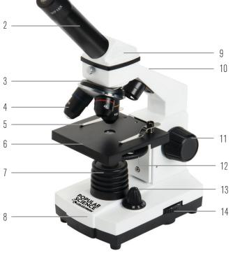
NOSEPIECE: Triple with click stop ILLUMINATOR: LED, adjustable CONDENSER: N.A. 0.65
