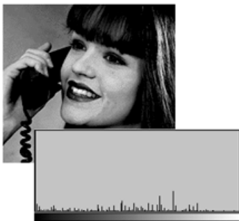
Figure 13. A high-contrast image. Gray levels are being spread out across the entire histogram.
