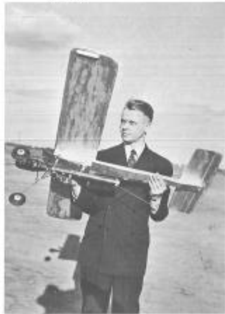
First known Dyno-jet powered flying model was this control-line shown here. The big model, with much metal, weighed 5 lbs. Developed by Bill Terry.
