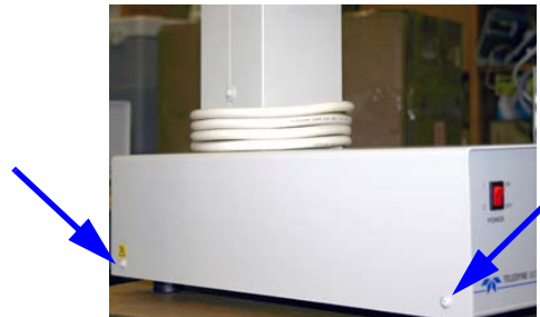
Figure 4: Pump case top screws (2 of 4 shown)
