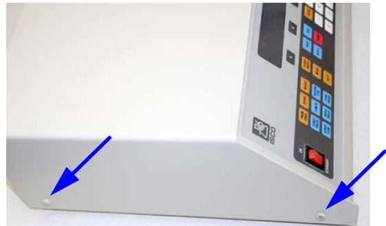
Figure 3: Controller case top screws (2 of 4 shown)
