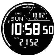
Display example (Upper display area: Barometric pressure, Lower display area: Altitude)
