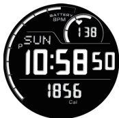
Display example (Upper display area: heart rate, Lower display area: Calories Burned)
