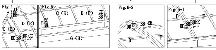
**Fig.4:** Insert Top Frame 1(C) into Top Frame 2 (D). Use Bolt (AA) and Washer (BB) to fix-up. Then use Bolt (CC), Washer (BB) and Nut (DD) to lock tight. Use the same method to attach Top Frame 3 (E) to Top Frame 4 (F).
