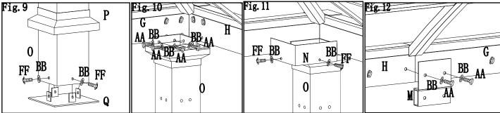
Fig.9: Lift up Stake Lid (P) firstly, then use Bolt (FF) and Washer (BB) to fix Stake Flake (Q) to Column (O).
