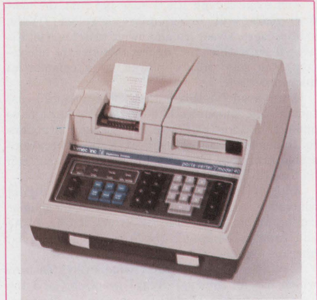
This remote data-entry terminal—the Porta-verter from Iomec, Inc.—offers intelligent operation. Credit goes to a four-bit microprocessor.
