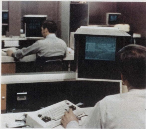
Four interactive graphics terminals, each linked to its own minicomputer, help design electronic circuits with Applicon's system. The host, also a mini, provides additional support for this star configuration and can act as a front-end to an IBM 360, which calculates the PC art-work routings.
