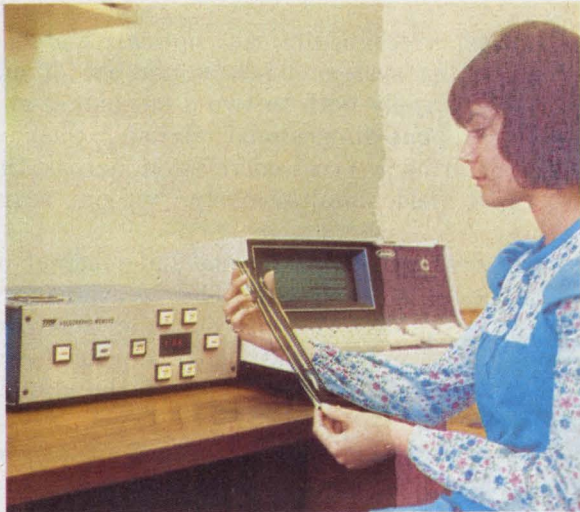
Holographic data retrieval unit from TRW is used to read data stored on 35 mm film. A separate holographic recorder is used to store data.
