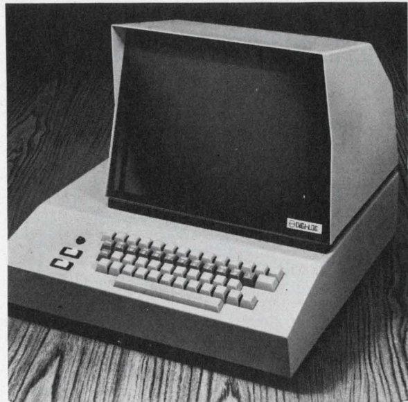
The Microterm series, built by Digi-Log Systems, are microprocessor-based, intelligent terminals that can be customized to a user's specs.
