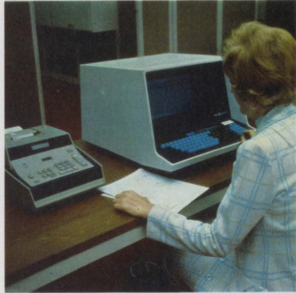
Sanders 810 intelligent terminal has a 12-in. cathode-ray tube with 1920 characters. It can support up to eight "dumb" terminals with its processor, and it sells for $6900.
