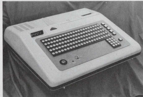
Staid Corporation's Datacash —a microprocessor-based point-of-sale terminal for restaurants—keeps an inventory of every key strike.
