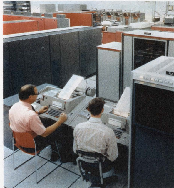
The Collins C-System uses a localized high-speed ring to join hosts and storage devices. Low-speed loops drive terminals and input devices. The system shown provides a statewide Iowa police network, with access to more than seven million traffic records and 250,000 criminal records on file in a System/370 complex at Des Moines.
