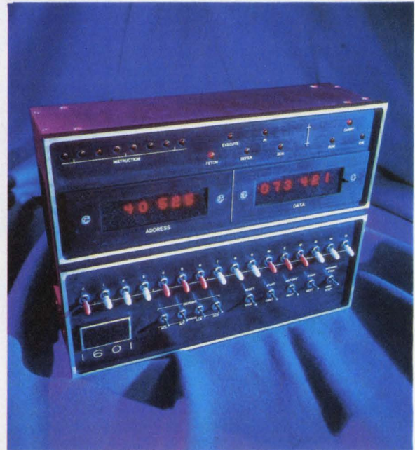
For harsh environments, Rolm minicomputers, produced to MIL specs, offer up to four times the MTBF of commercial counterparts.
