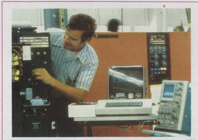
The finished product tests other System/7's at IBM before shipment. The System/7 under test (left) is linked to the computer that monitors memory operation, control functions and data flow. Test data are printed out on a console (right, background) and relayed to a central System/360. A single System/7 can test up to four processors.
