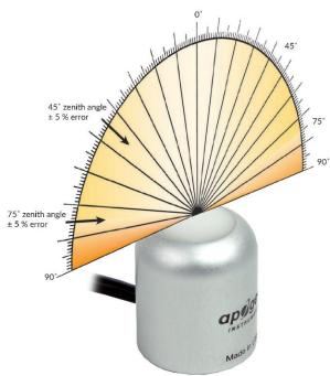
Directional, or cosine, response is defined as the measurement error at a specific angle of radiation incidence. Error for Apogee SQ-600 series Extended Range PFD Sensor is approximately  $\pm 2$  % and  $\pm 5$  % at solar zenith angles of 45° and 75°, respectively.
