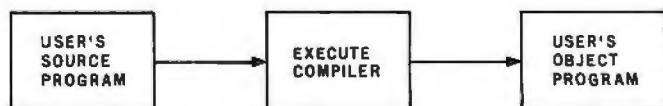
Figure 1: Compilation of any computer language. A program in some computer language is input to a compiler. The compiler produces a functionally equivalent program in a different, object language.
