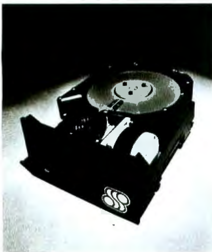
Photo 3: The remarkable Shugart Technology Model ST506 hard-disk drive, offering 6 megabytes of mass storage in a 3.5-pound package that fits in the same space as a 5-inch floppy-disk drive. (Shugart Technology is a new company located in Scotts Valley, California, and is not affiliated with either Shugart Associates or Xerox. Photo courtesy of Shugart Technology.)
