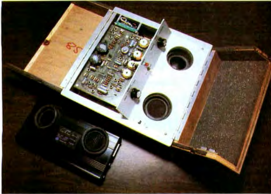
Photo 2: Comparison of two generations of modems. At right is an early model made by Anderson-Jacobson, shown with the covers open. The old modem uses discrete semiconductor components and toroidal inductors. On the left is an example of a current model of modem: a Novation Cat acoustic-coupled modem, which is popular with home-computer hobbyists.
