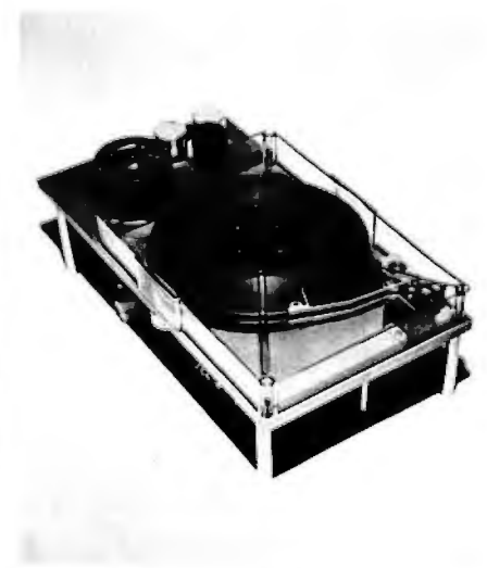
Photo 6: Kennedy Series 7000 8-inch hard-disk drive. (Photo courtesy of Kennedy Company.)
