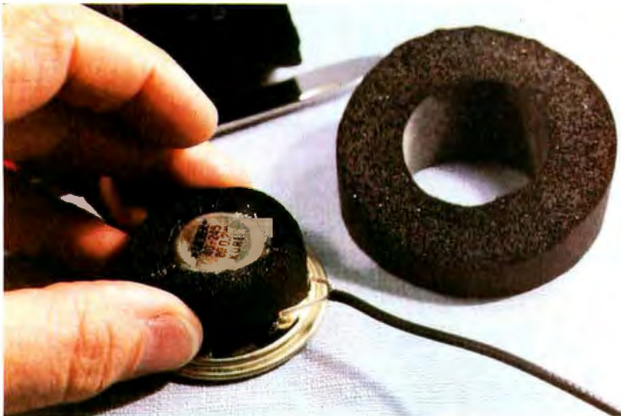
Photo 3: First of a series of photos (3 thru 9) showing how you can easily construct an acoustic-coupler pickup. My design for the pickup uses such "exotic" materials as a hot-water pipe foam insulation, a pair of 2-inch, 8-ohm dynamic speakers, a foam-backed dinner placemat, rubber cement, and adhesive tape.
