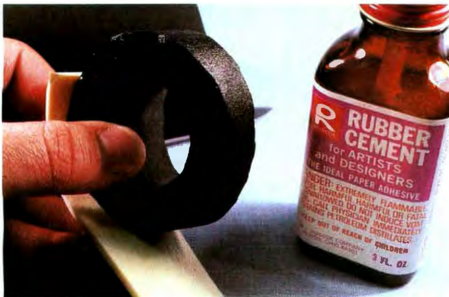
Photo 5: Adding pliable material to produce a tight fit around the phone handset. I found a plastic placemat at a discount store with a 1/8-inch foam backing that was perfect. Cut a strip 1 1/2 by 8 inches and glue this around the outside of the wedge as shown. Trim to the exact circumference and cover with a strip of fabric adhesive tape. The latter helps hold everything together.
