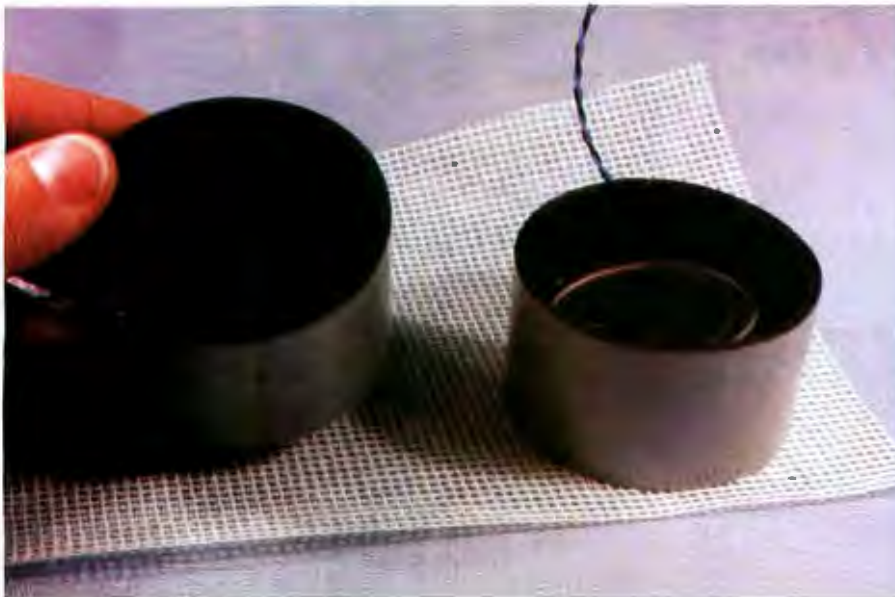
Photo 8: The final assembly can be spray-painted black as I have done, but this is not necessary. Caution: some paints act as solvents on foam and will produce a sticky mess. Test a small sample before spraying the whole unit, and don't spray the speaker cone.
