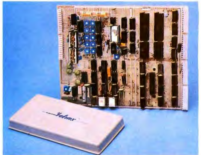
Photo 1: The CA-15 universal telephone interface board, shown with its optional Votrax voice synthesis module.
