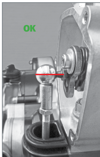
Correct position of the control rod seat.
