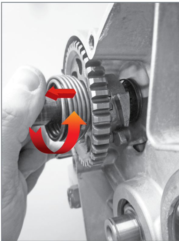
Extraction of shaft from crankcase.
