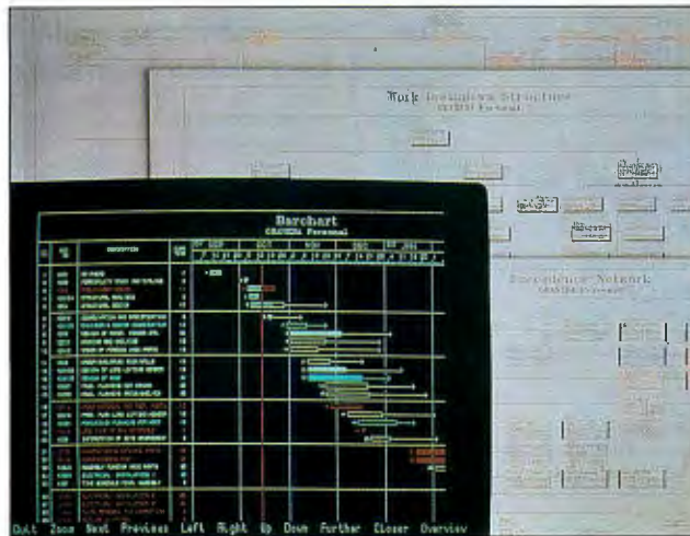
The four types of drawings that Graneda can create include precedence network, arrow network, bar charts, and work breakdown structures.
