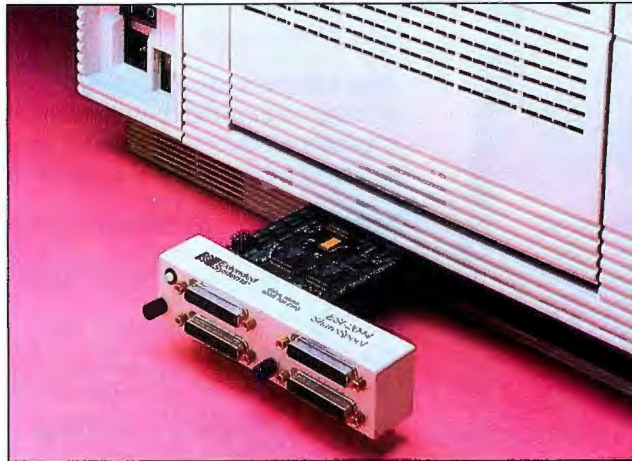
ShareSpool cards connect your LaserJet to as many as four computers. They also provide RAM for spooling.
