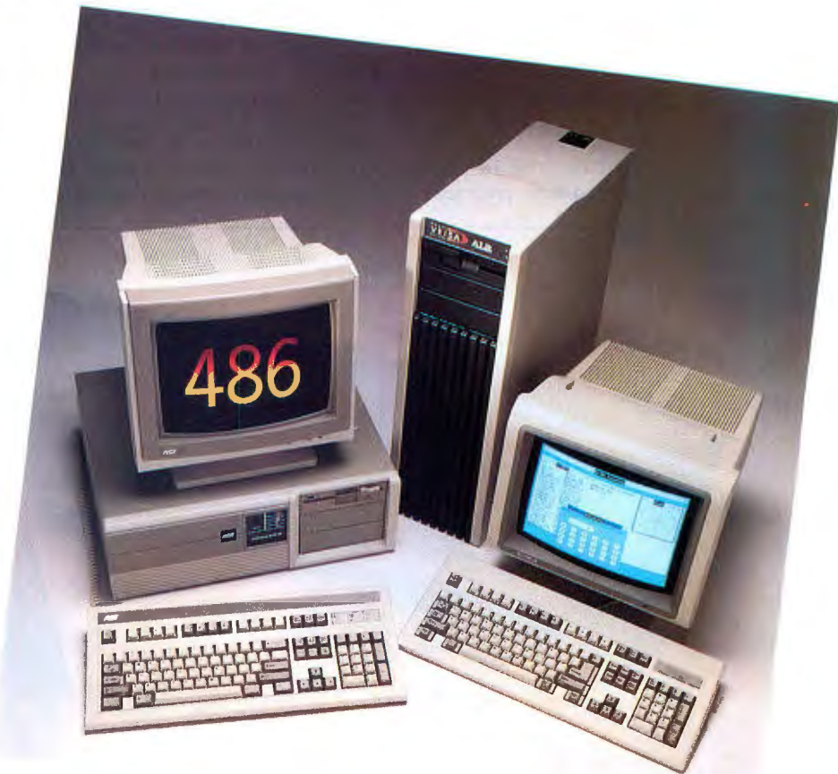
Photo 1: The AST Premium 486/33 (left) is a desktop design with an ISA bus, while the ALR PowerVEISA 486/33 sports a tower design with an EISA bus. AST offers EISA versions in both desktop and tower form.
