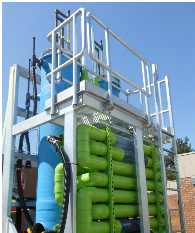
IMAGE 3: Plug-flow reactors treat effluent at 15 gallons per minute
