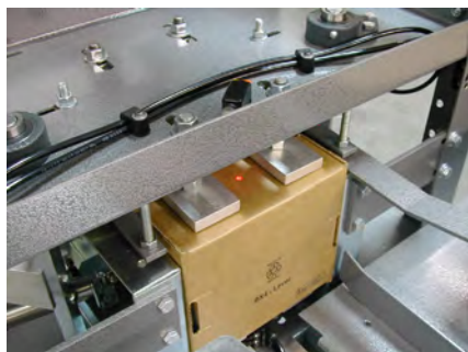
FIGURE 2: The completed tray is positioned at the machine output on its side for easy stacking with other trays.
