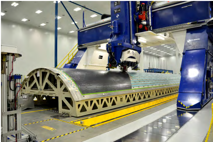
FIGURE 1: Electroimpact's Automated Fiber Placement technology is used to create fuselage panels for the Airbus A350 aircraft. (Image courtesy of Electroimpact).
