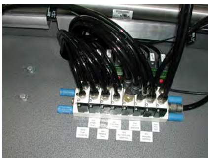
FIGURE 3: Air valves and a manifold provide fluid power to the cylinders that feed, assemble and stack the trays.
