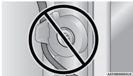
Incorrectly Seated Tailgate Strap
