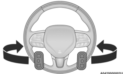
Remote Sound System Controls
