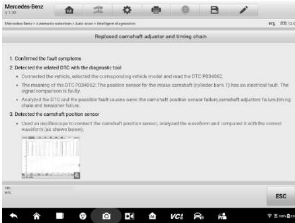
Figure 5-23 Sample Repair Tips Description 1 (Text)
