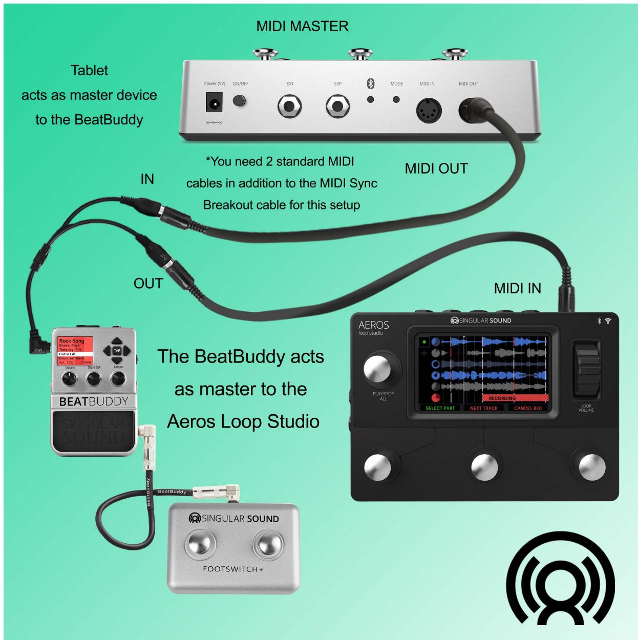
**A typical configuration using both the IN and the OUT ports on the MIDI Sync Breakout cable at once. (Beatbuddy set to MIDI Merge see Section 8 MIDI and the BeatBuddy)**
