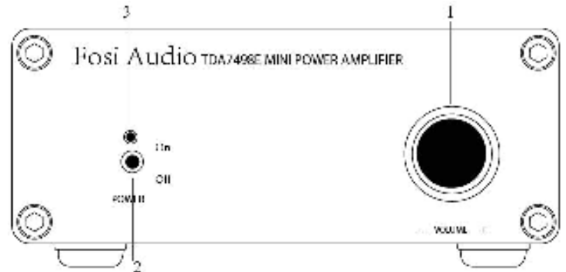
1..... Volume Control 3..... Power Indicator 2..... Power Switch
