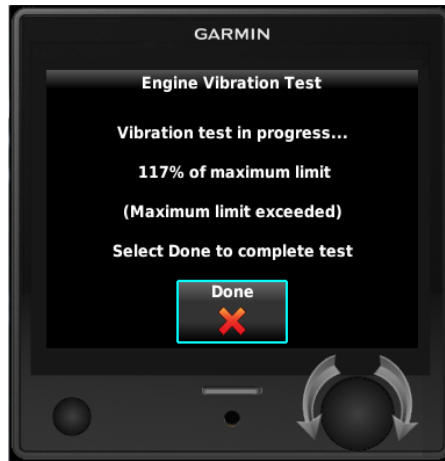
Figure 6-3 Engine Vibration Test Failure Indication
