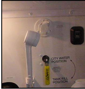
Figure 11-7. City Water Supply Connection
