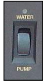
Figure 11-5. Water Pump Switch
