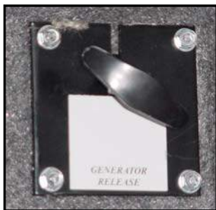
Figure 7-18. Generator “Pull” Cable Slide-Lock Release
