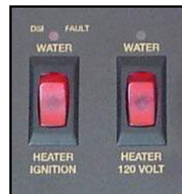
Figure 4-17. Water Heater Switches
