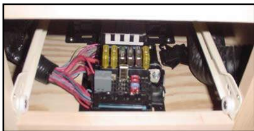
Figure 7-21. Fuse Blocks within Center Console
