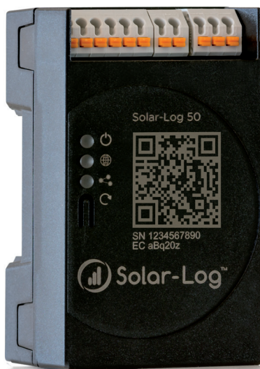
Fig.: Gateway Solar-Log 50 without extended snap-fit tabs
