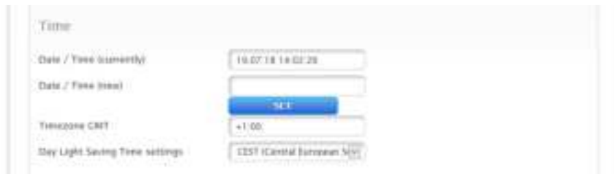
Fig.: Configuring the time on the Solar-Log™
