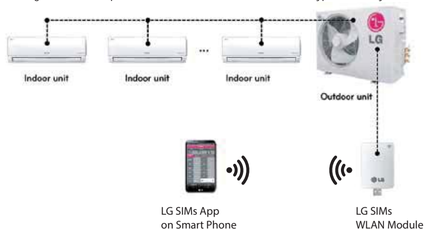
Figure 137: Example of a SIMS WLAN Module Used with a Typical DFS System.
