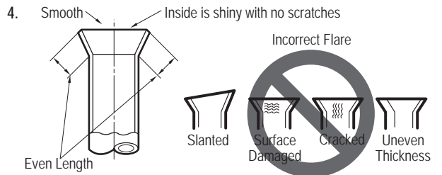
Flared Connection Dimensions / Tightening Torque.
