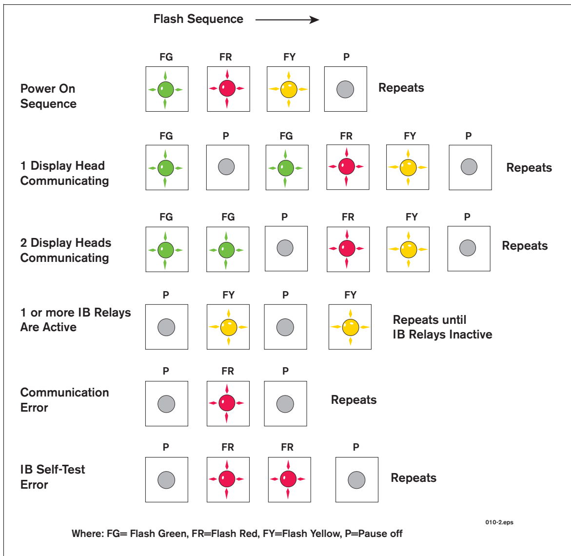
Figure 2. IB Tri-Color LED Status Patterns
