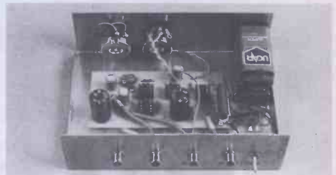
The circuit is powered by two PP3 batteries. All of the inputs and outputs are available on the rear panel. They are from left to right: X', 'Y', OUT and OSC.
