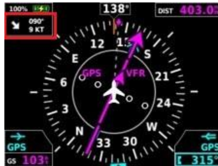
Figure 6-5 HSI Display of Crosswind (Typical Values Shown)
