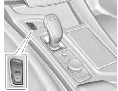
Driver Mode Control Switch
