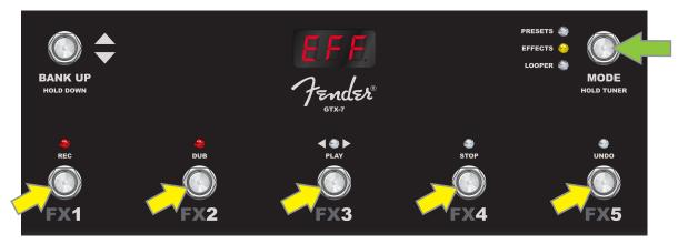
EFFECTS mode example showing a preset with two effects, each assigned to FUNCTION buttons FX1 and FX2. The illuminated red FUNCTION LEDs above FX1 and FX2 indicate that both effects are on; both can be turned off by stepping on their respective FUNCTION buttons.
