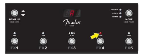
Here, the "A" note is displayed as being slightly sharp, as indicated by the illumination of FUNCTION LED 4 (yellow arrow).
