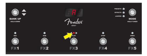
Here, the "A" note is at correct pitch, as indicated by the illumination of FUNCTION LED 3 at center (yellow arrow). When tuning is complete, step on any button to exit footswitch tuner mode.
