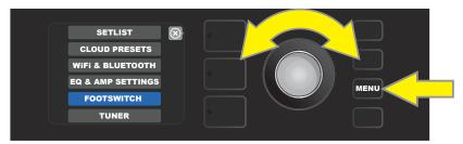
Use the ENCODER to scroll to and select "GTX-7 (7-BUTTON)" from the menu of devices shown, then use the ENCODER to scroll to and select "FX ASSIGN":
