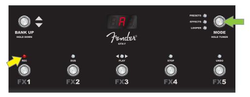
To activate the GTX-7 Footswitch tuning function, step on and briefly hold the MODE button (green arrow). In the example shown here, an "A" note is displayed as being particularly flat, as indicated by the illumination of FUNCTION LED 1 at far left (yellow arrow).
