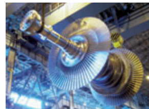
High-efficiency turbine for thermal power generation
