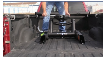
Attach the hitch head.
