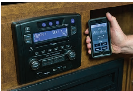
(Above left) Outside features include a 120-volt AC receptacle and a cable-TV connection aft of the rear door. (Above right) The iRV Technologies DVD-stereo system has three speaker zones and allows control through the receiver panel or an app on Bluetooth-enabled devices. The receiver contains a CD/DVD drive, an SD-card slot, and USB and HDMI ports.
