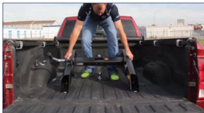
BXR6200: attach the base to a 2-5/16" gooseneck hitch or to rails for model BXR7200.
