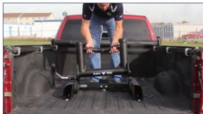
Slide the shock towers into the base.
