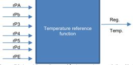
It's possible to set the probes used for temperature regulation. Up to 5 Temperature inputs Pb1, Pb2, Pb3, Pb4, Pb6, can be used.
