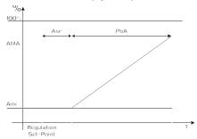
The modulating output (trA=rEG) works in proportional way (excluding the first AMt seconds where the fans speed is the maximum). The regulation set point is relative to regulation set point and is indicated by ASr, the proportional band is always located above SET+ASr value and its value is PbA. The fan are at minimum speed (AMI) when the temperature read by fan probe is SET+ASr and the fan is at maximum speed (AMA) when the temperature is SET+ASr+PbA.
