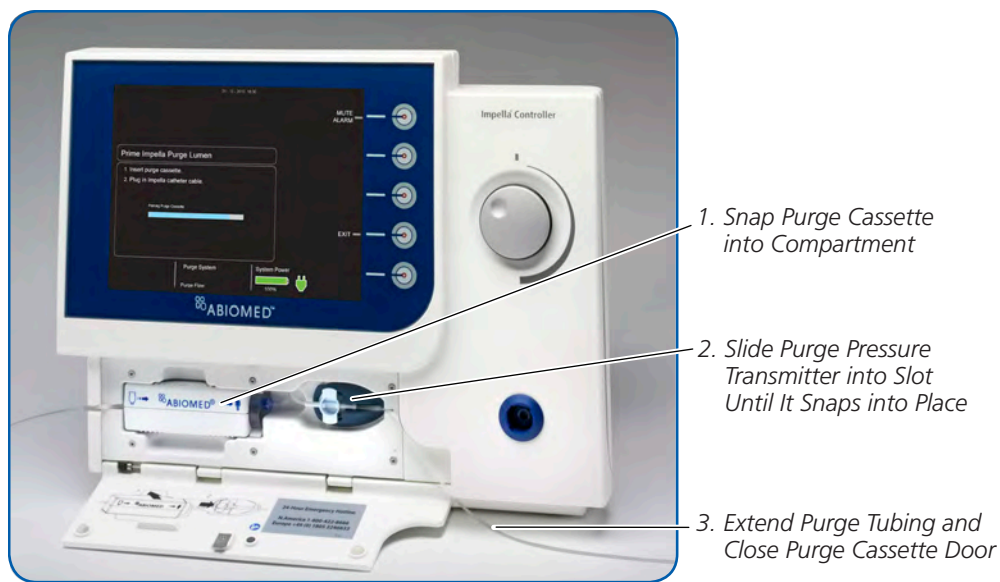
Figure 5.4 Inserting the Purge Cassette into the Automated Impella® Controller
