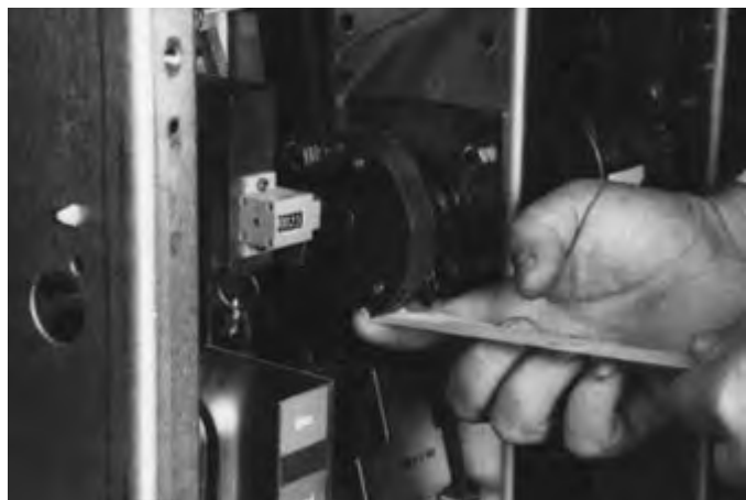
Figure 6-6 Starting Tape at Bottom of Cam
