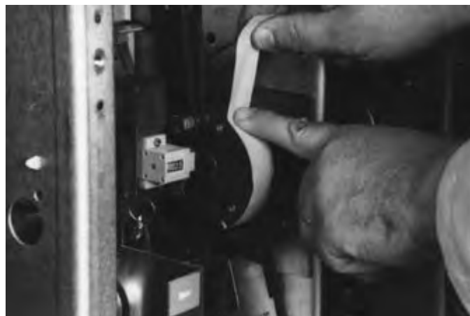
Figure 6-7 Wrapping Tape Up Around Cam
