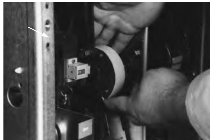
Figure 6-8 Attaching Tape Around to Back of Cam
