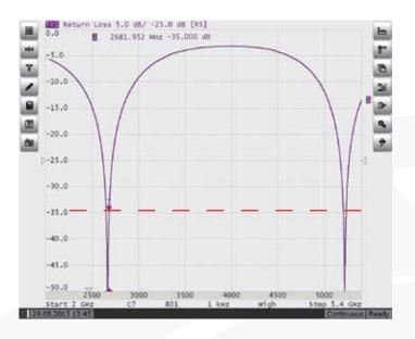
R54 and R60 can measure return loss up to 35 dB in their entire frequency range. R140 can measure return loss up to 35 dB from 85 MHz to 4.8 GHz and 25 dB from 4.8 GHz to 14 GHz. R140, which is a specification typical of benchtop instrumentation.
