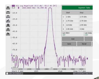
Reflectometers have a large frequency range with the option of frequency scan segmentation. This allows the user an opportunity to use the reflectometer, for example, to realize the maximum dynamic range while maintaining high measurement speed.
