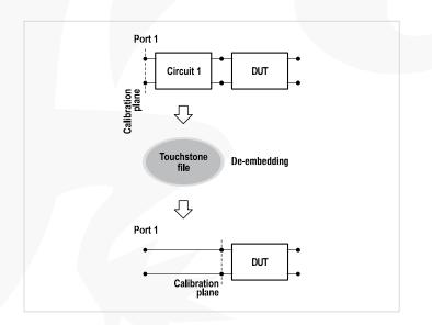
The function allows to mathematically exclude from the measurement result the effect of the fixture circuit connected between the calibration plane and the DUT. This circuit should be described by an S-parameter matrix in a Touchstone file.
