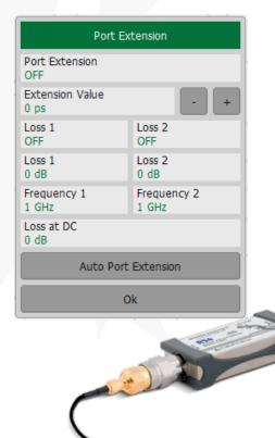
Port Extension is a feature that allows for moving the calibration reference plane of the port by specifying the electrical delay to the new reference plane position. Additionally, it is possible to account for loss in the extended port.
