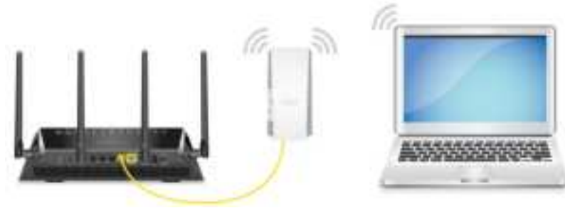
Figure 4. Extender in access point mode
