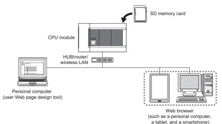
Use a straight cable with either of the following specifications. If a personal computer is to be directly connected to a CPU module with an Ethernet cable, a cross cable whose specification is category 5e or less can be used.
