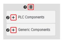
Click the symbol on the right side of ① to fold a component window in question. If a component window is folded, click such a symbol to unfold it. Click the symbol on the right side of ② to fold a corresponding PLC/generic component's list. If such a list is folded, [ - ] will appear on the right side of ②. Click [ - ] to unfold such a list in question.
