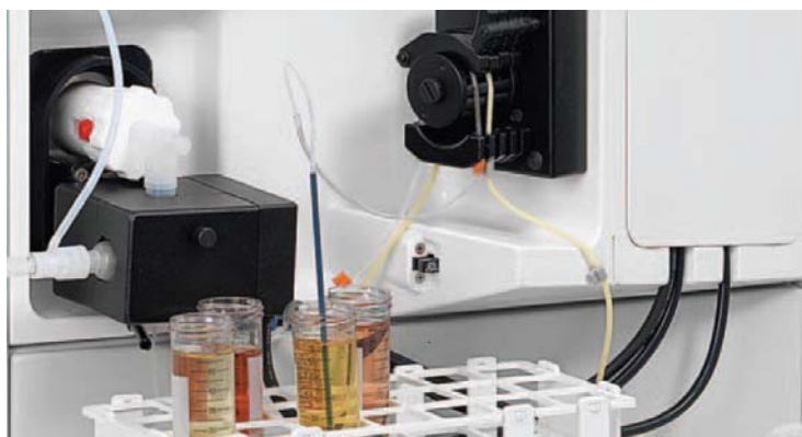
Figure 3-4. Peristaltic pump at inlet system
