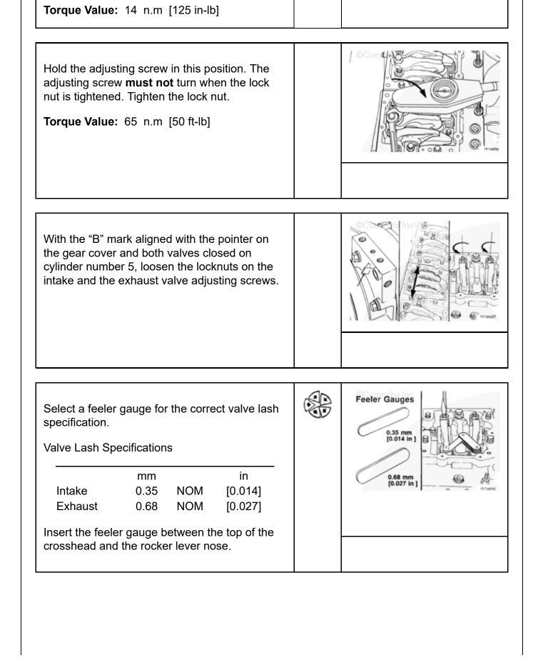
Two different methods for establishing valve lash clearance are described below. Either method can be used: however, the torque wrench method has proven to be the most consistent.
