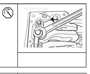
After setting the injector on a given cylinder, set the valves on the same cylinder.
