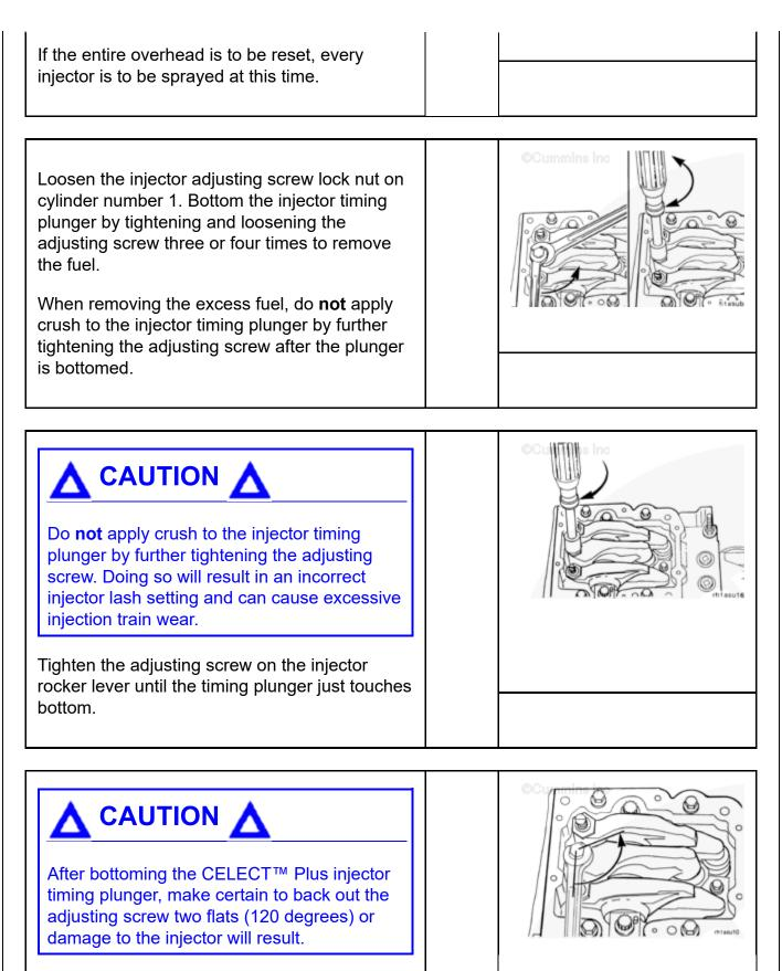
Back out the adjusting screw on the injector rocker lever two flats (120 degrees).
