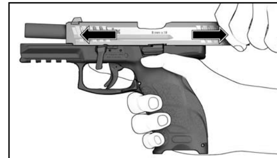
Figure 15 — Removing slide from frame by pushing it forward
