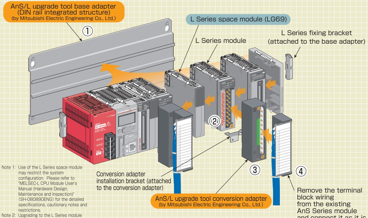
Note 1: Use of the L Series space module may restrict the system configuration. Please refer to "MELSEC-L CPU Module User's Manual (Hardware Design, Maintenance and Inspection)" (SH-080890ENG) for the detailed specifications, cautionary notes and restrictions.
