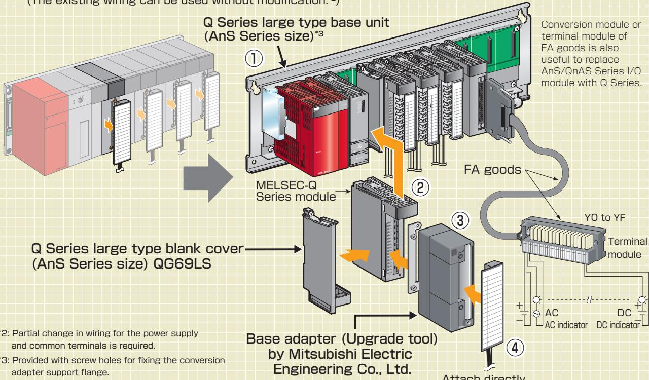
\*2: Partial change in wiring for the power supply and common terminals is required.
