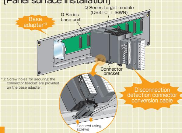
\*3: Screw holes for securing the connector bracket are provided on the base adapter.
