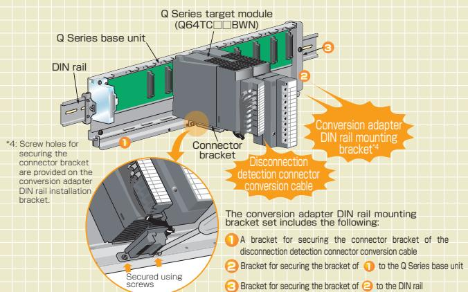
\*4: Screw holes for securing the connector bracket are provided on the conversion adapter DIN rail installation bracket.
