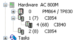
Figure 9. Redundant CI840 in HW-Tree
